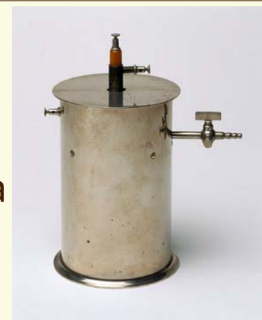
Ionization chamber made by Pierre Curie, c 1895-1900
