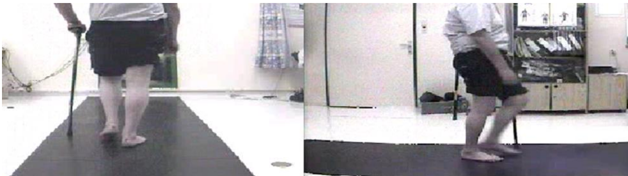
Figure N2. Force measuring track for capturing the gait cycle in the specialized walk-investigating laboratory
