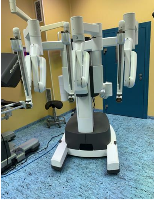
Figure 5. System for robotic surgery DaVinci X.
